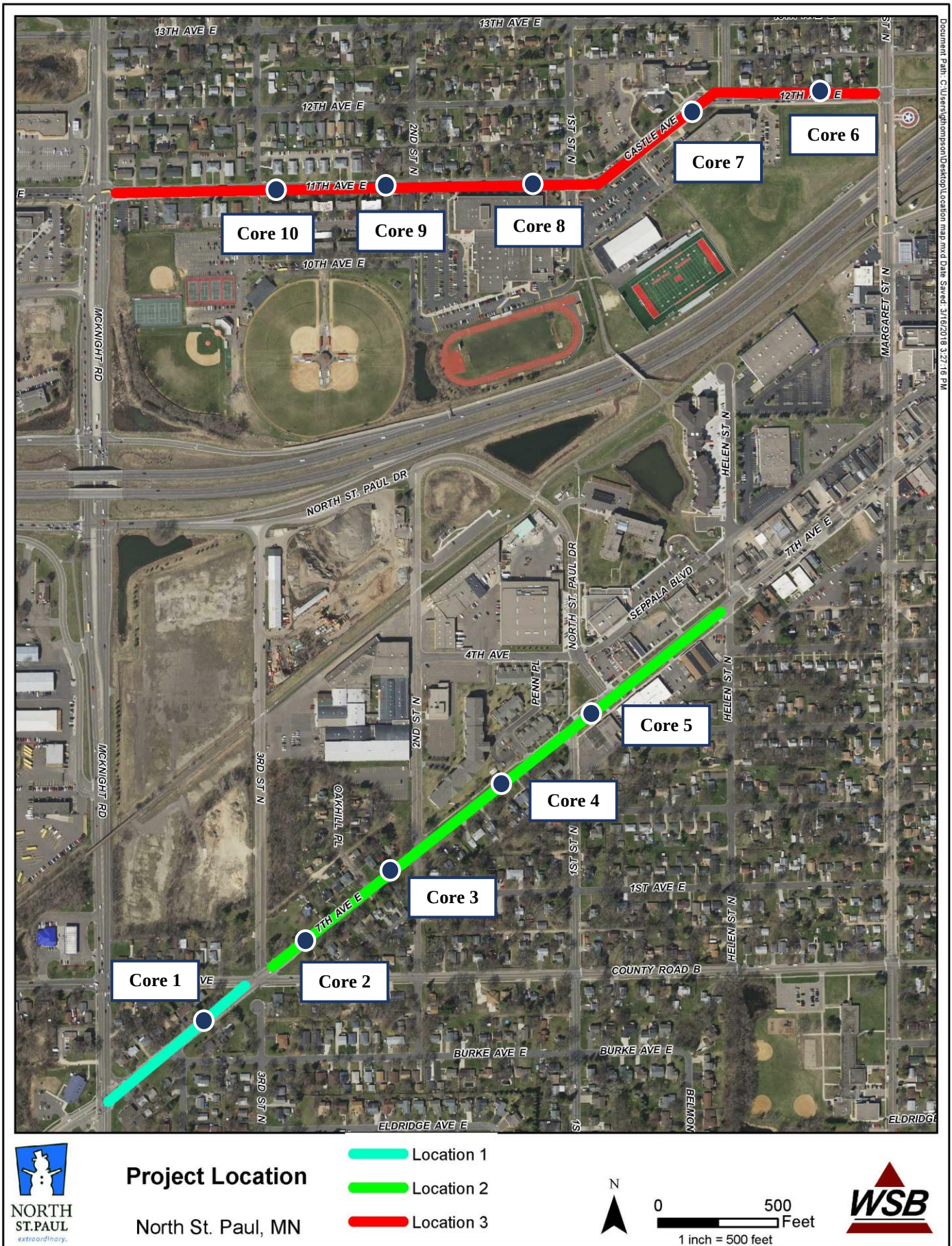
Figure 1. Pavement core locations taken within the City of North St. Paul.
