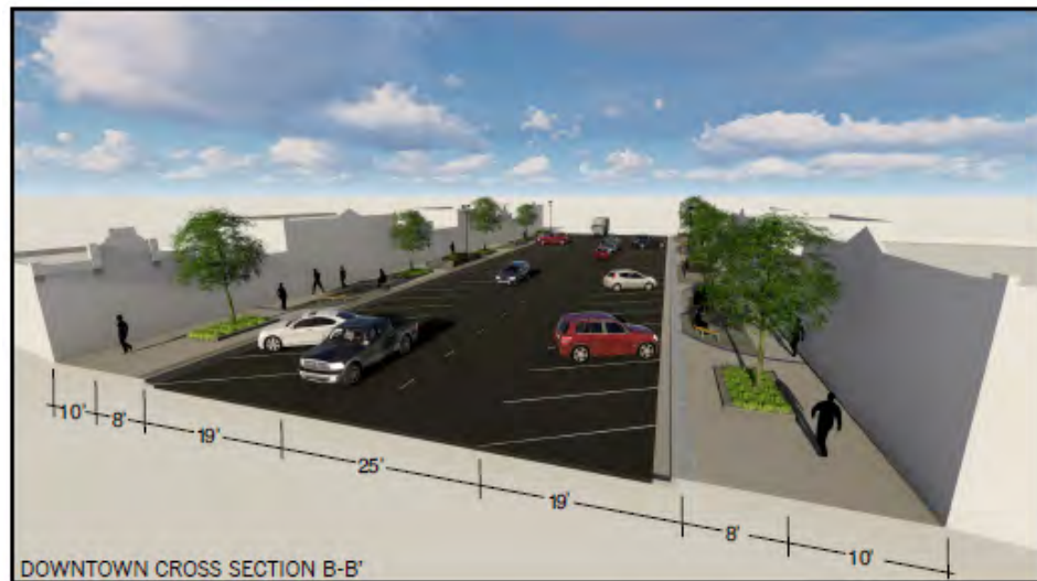
FIGURE 7-5 CROSS SECTION OF DOWNTOWN CORE AREA
