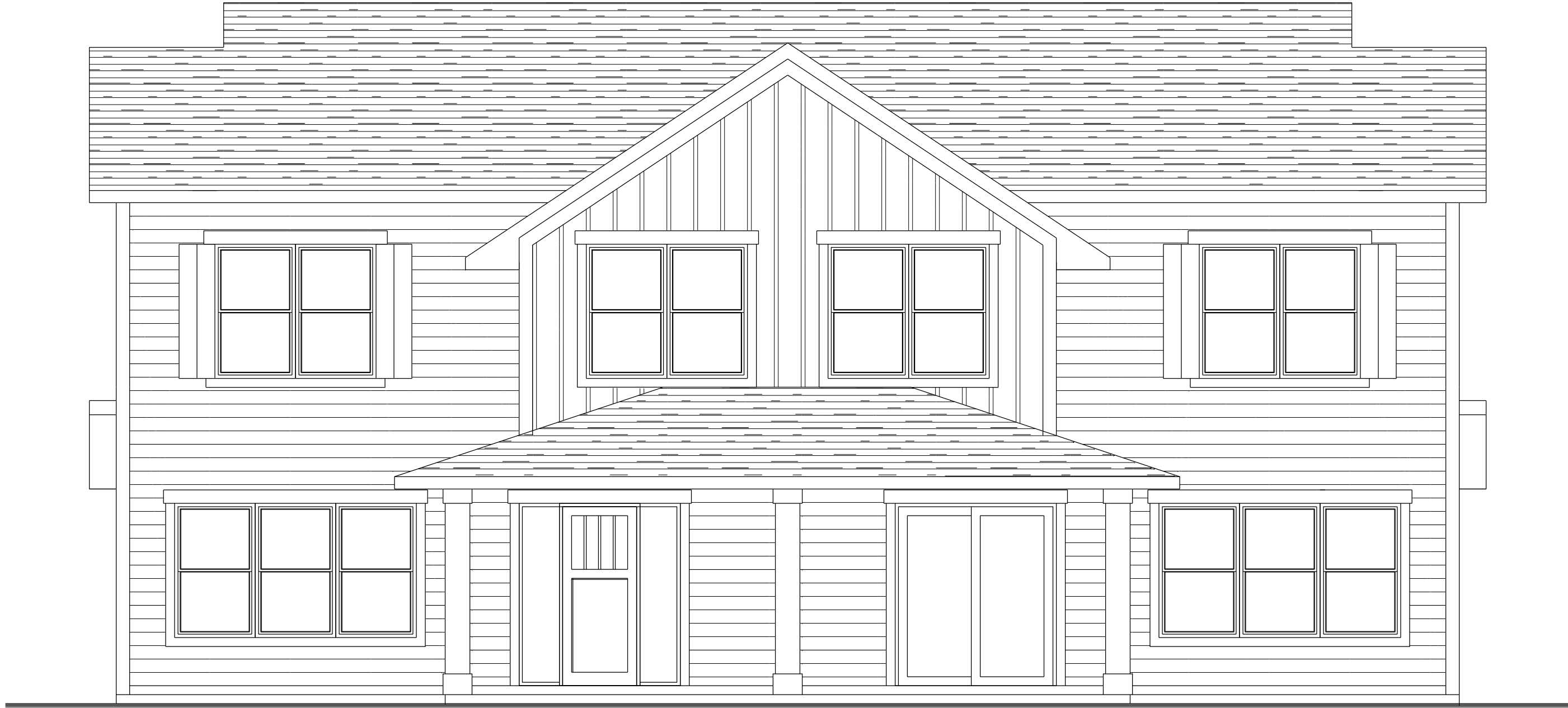
REAR ELEVATION W/ COVERED PORCHES B SCALE 1/4" = 1'-0"
