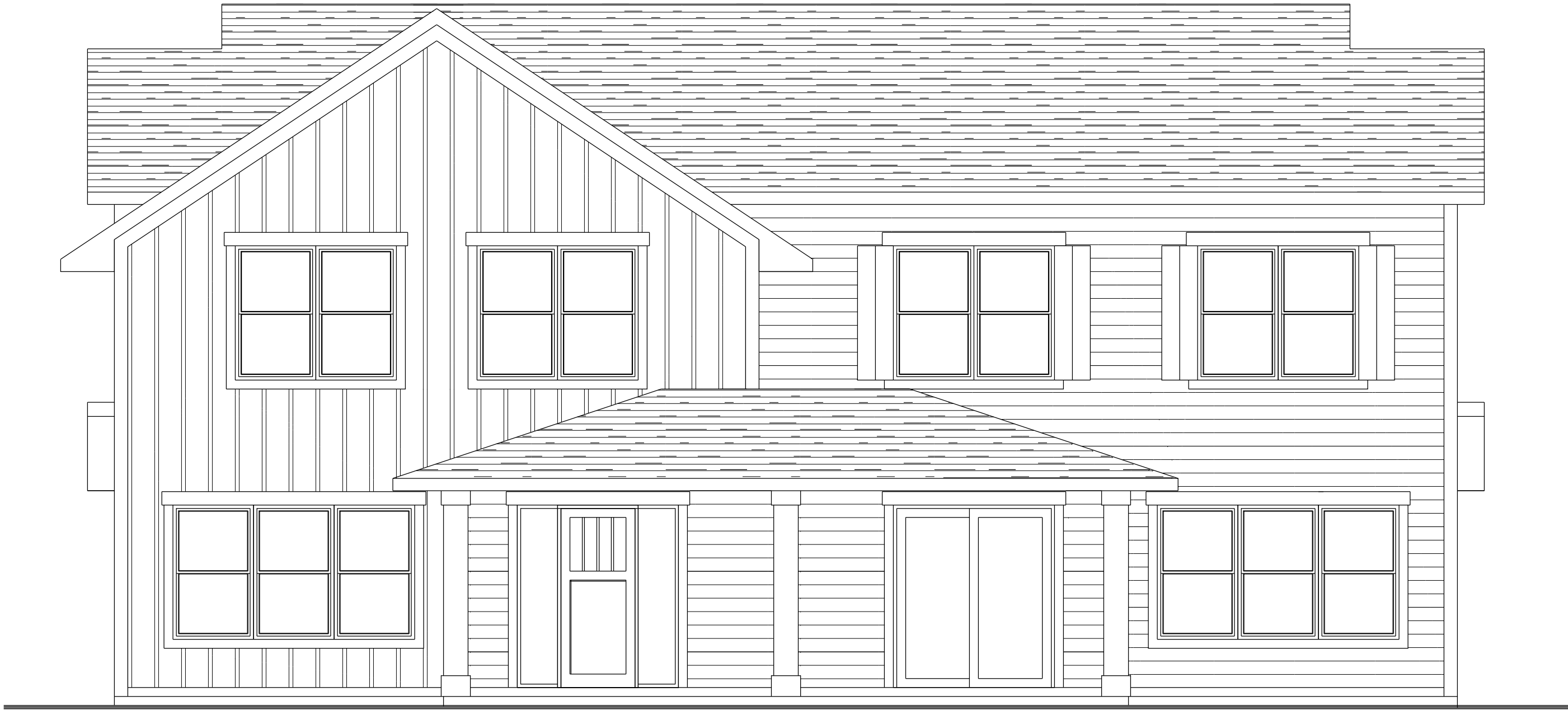
REAR ELEVATION W/ COVERED PORCHES C SCALE 1/4" = 1'-0"
